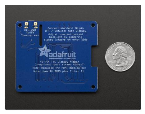
Comes as one fully assembled and tested DPI Kippah circuit board. You may need a soldering iron to adjust the backlight by soldering closed a PCB jumper (check the tutorial on this). TFT display (https://adafru.it/Cfx), USB micro-B cable (http://adafru.it/
