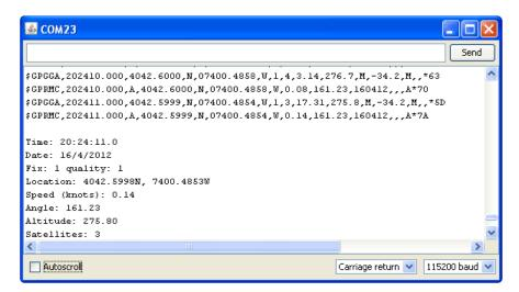
In this sketch, we call GPS.read() constantly in the main loop (if you can, get this to run once a millisecond in an interrupt). Then in the main loop we can ask if a new chunk of data has been received by calling GPS.newNMEAreceived(), if this returns true then we can ask the library to parse that data with GPS.parse(GPS.lastNMEA()).
