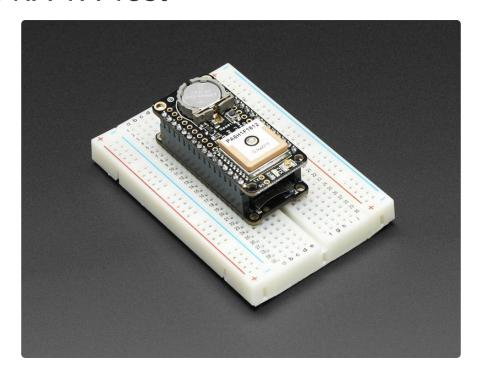
The first, and simplest test, is just to echo data back and forth using the Feather's USB connection to read the GPS data out. The nice thing about this demo is no library is required.
