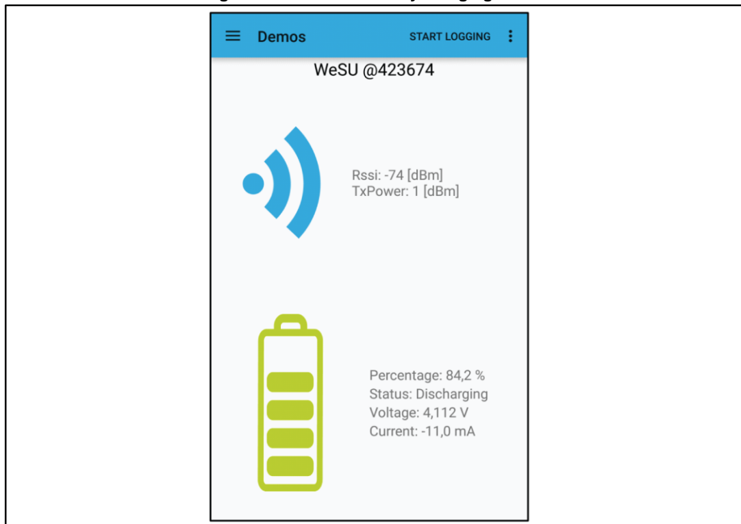
Figure 62: RSSI and battery charging demo
