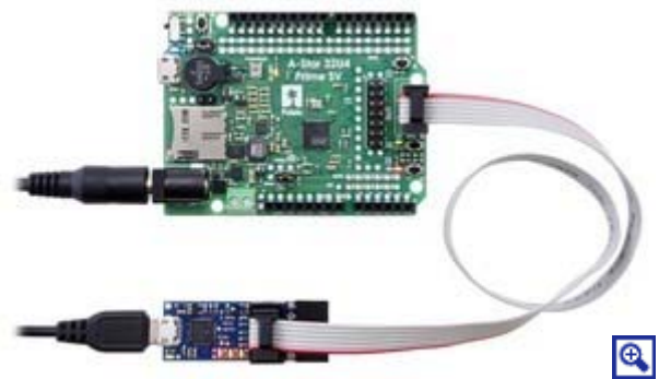
The Pololu USB AVR Programmer v2 (bottom) connected to an A-Star 32U4 Prime SV for programming.
