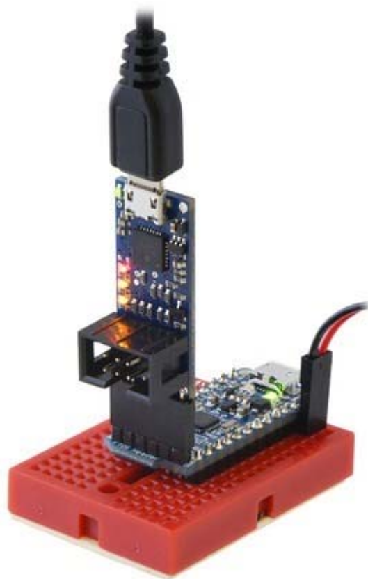
The Pololu USB AVR Programmer v2 (top) connected to an Adafruit Pro Trinket for programming.
