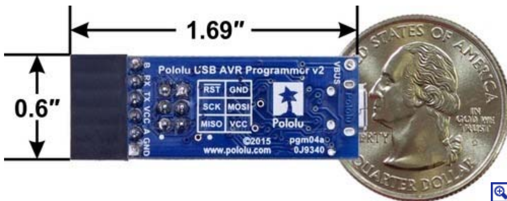
Pololu USB AVR Programmer v2, bottom view with dimensions.
