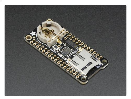
This FeatherWing will make it real easy to add datalogging to any of our existing Feathers. You get both an I2C real time clock (PCF8523) with 32KHz crystal and battery backup, and a microSD socket that connects to the SPI port pins (+ extra pin for CS). Tested and works great with *any* of our Feathers, based on ATmega32u4, ATmega328P, ATSAMD21, ATSAMD51, nRF52, Teensy, or ESP32/ESP8266.
