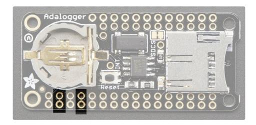
On the bottom row, the **3.3V** (second from left) and **GND** (fourth from left) pin are used to power the SD card and RTC (to take a load off the coin cell battery when main power is available)
