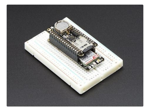
But don't forget, you can also put the stacking headers on the wing and stack the Feather on top of it!
