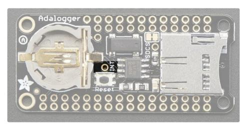
There's also a breakout for **INT** which is the output pin from the RTC. It can be used as an interrupt output or it could also be used to generate a square wave.
