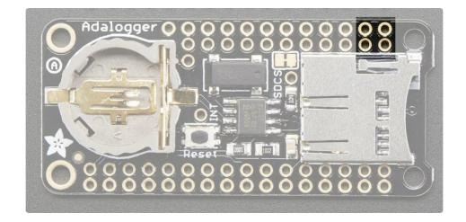
In the top right, SDA (rightmost) and SCL (to the left of SDA) are used to talk to the RTC chip.
