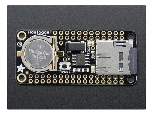
A Feather board without ambition is a Feather board without FeatherWings! This is the **Adalogger FeatherWing**: it adds both a battery-backed Real Time Clock and micro SD card storage to any Feather main board. Using our <u>Feather Stacking Headers</u> (http://adafru.it/2830) or <u>Feather Female</u> <u>Headers</u> (http://adafru.it/2886) you can connect a FeatherWing on top of your Feather board and let the board take flight!
