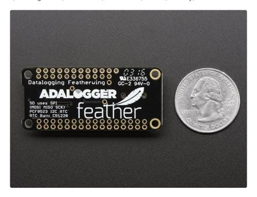
We recommend the Arduino's default SD library to talk to the microSD card socket. On ESP8266, the SD CS pin is on GPIO 15, on Atmel M0, M4, 328P or 32u4 it's on GPIO 10. You can cut the trace to the default pin and change this to any pin. To use the RTC, <u>use our RTClib library</u> (https://adafru.it/c7r). If you need a <u>precision RTC, check out our DS3231 FeatherWing</u> (http://adafru.it/3028)
