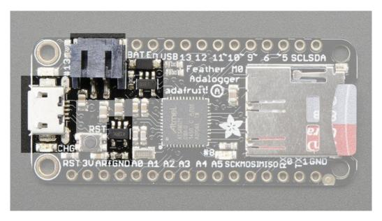
The above shows the Micro USB jack (left), Lipoly JST jack (top left), as well as the 3.3V regulator and changeover diode (just to the right of the JST jack) and the Lipoly charging circuitry (to the right of the Reset button). There's also a **CHG** LED, which will light up while the battery is charging. This LED might also flicker if the battery is not connected.
