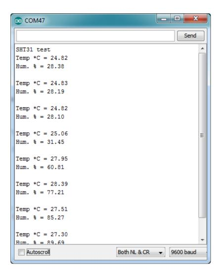
You can try breathing on the sensor to increase the humidity. The sensor reacts very fast!
