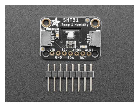
Unlike earlier SHT sensors, this sensor has a true I2C interface, with two address options. It also is 3V or 5V compliant, so you can power and communicate with it using any microcontroller or microcomputer.
