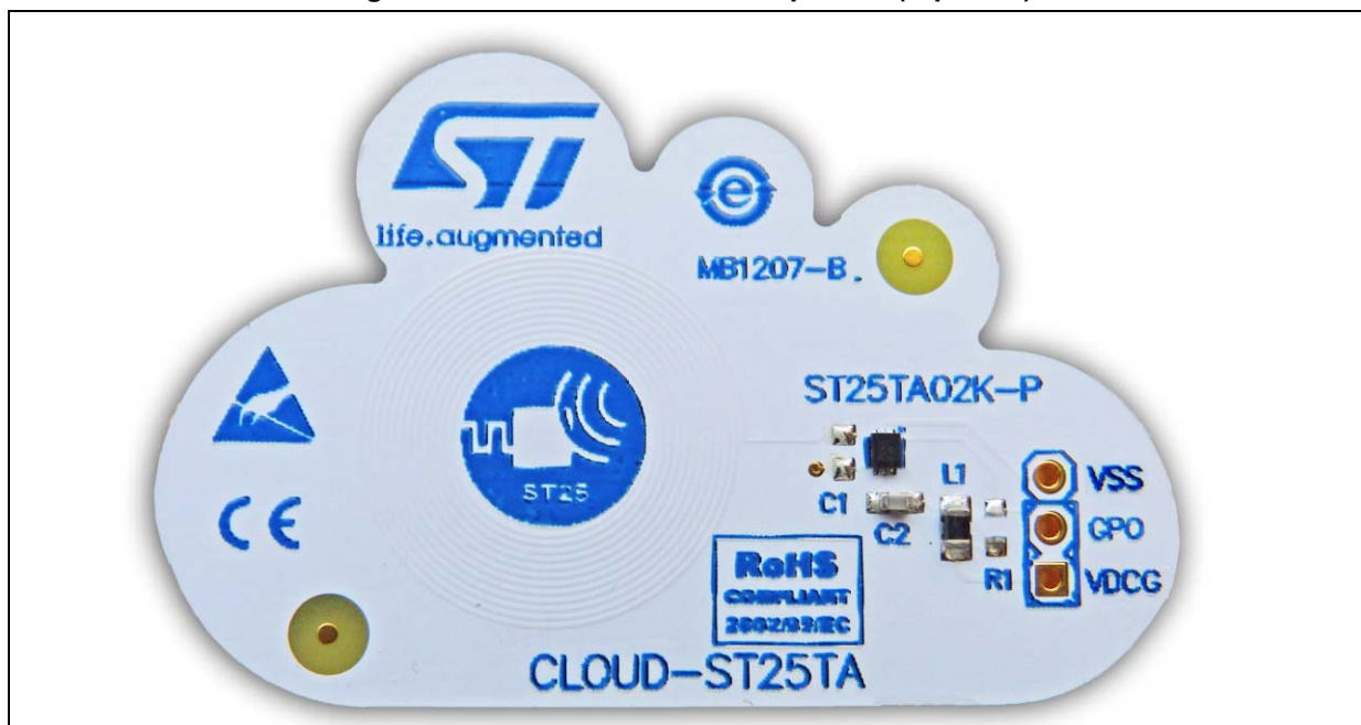
Figure 1. CLOUD-ST25TA board picture (top view)
