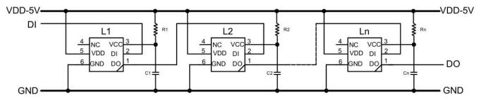
Remarks: **Rx** is the IC's protective resistance, power spike and reverse connection of the battery power terminal will be protected, its value is less than 100ohm. C1 is the bypass capacitor for VDD, its value of 100NF.
