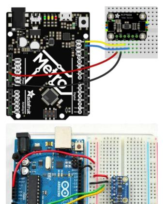
Connect VIN (Vdd) (red wire on the STEMMA QT version) to the power supply, 3V or 5V is fine. Use the same voltage that the microcontroller logic is based off of. For most Arduinos, that is 5V Connect GND (black wire on the STEMMA QT version) to common power/data ground
