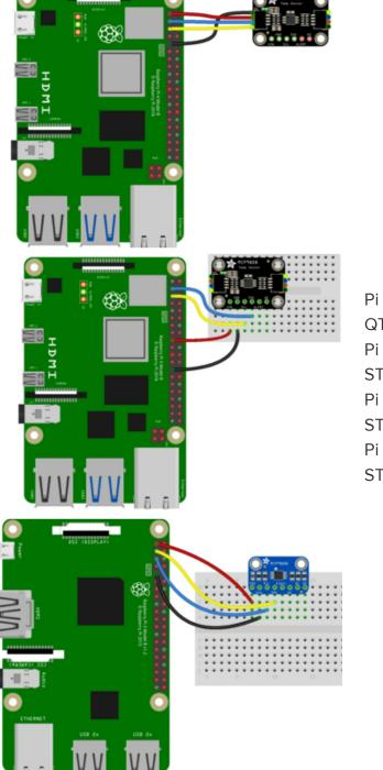
Pi 3V3 to sensor VIN (red wire on STEMMA QT version) Pi GND to sensor GND (black wire on STEMMA QT version) Pi SCL to sensor SCK (yellow wire on STEMMA QT version) Pi SDA to sensor SDA (blue wire on STEMMA QT version)
