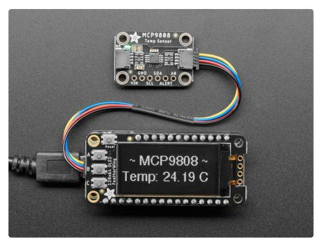
This I2C digital temperature sensor is one of the more accurate/precise we've ever seen, with a typical accuracy of ±0.25°C over the sensor's -40°C to +125°C range and precision of +0.0625°C. They work great with any microcontroller using standard i2c. There are 3 address pins so you can connect up to 8 to a single I2C bus without address collisions. Best of all, a wide voltage range makes is usable with 2.7V to 5.5V logic!
