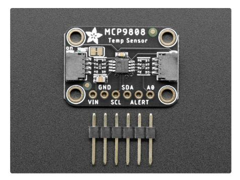
Unlike the DS18B20, this sensor does not come in through-hole package so we placed this small sensor on a breakout board PCB for easy use. The PCB includes
