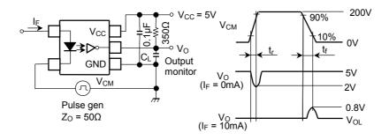
$${\sf CM}_{\sf H} = \frac{160({\sf V})}{t_{\sf \Gamma}(\mu {\sf s})}, {\sf CM}_{\sf L} = \frac{160({\sf V})}{t_{\sf f}(\mu {\sf s})}$$
