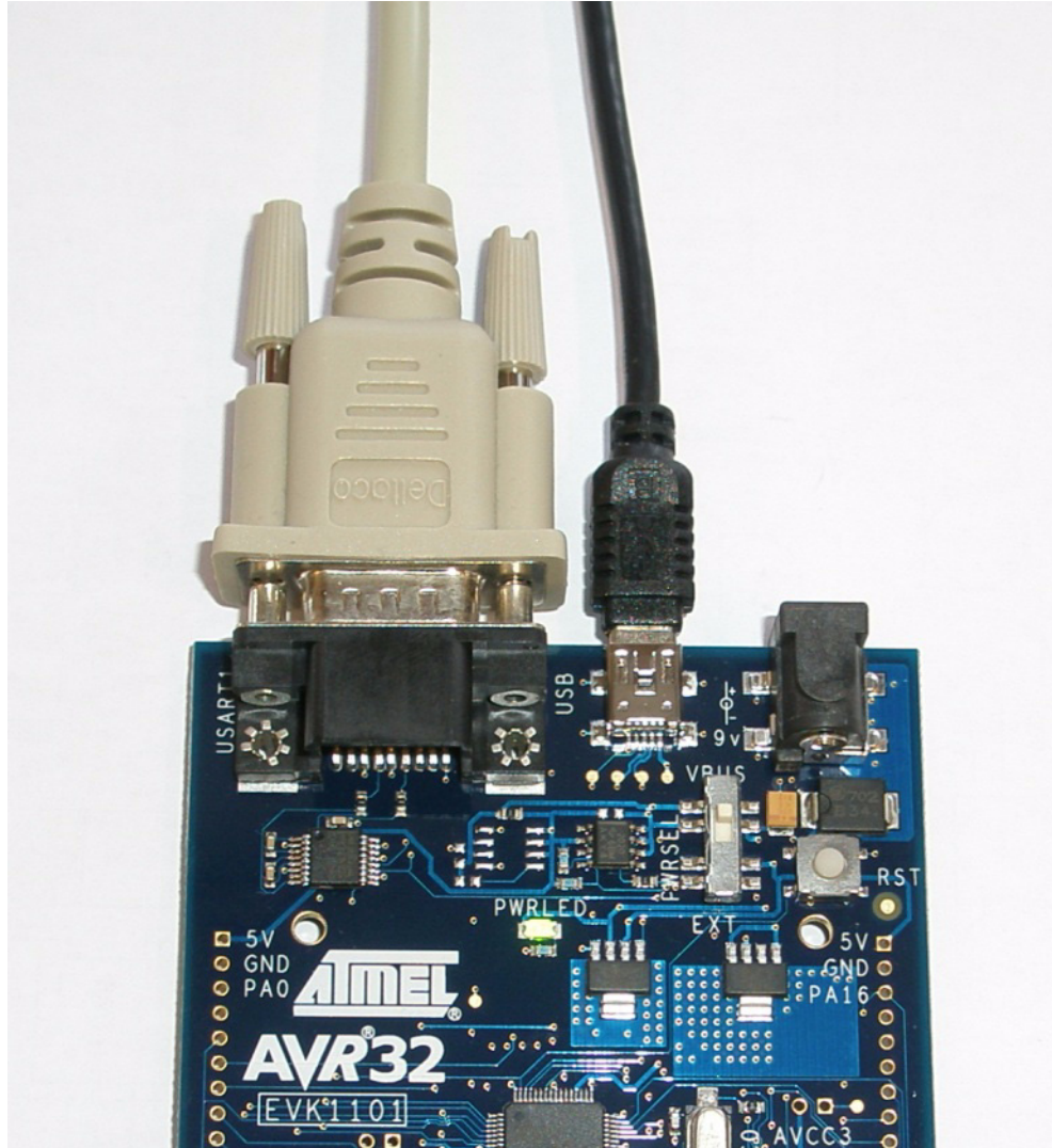
Figure 4-2. Powering the EVK1101 using the USB cable
