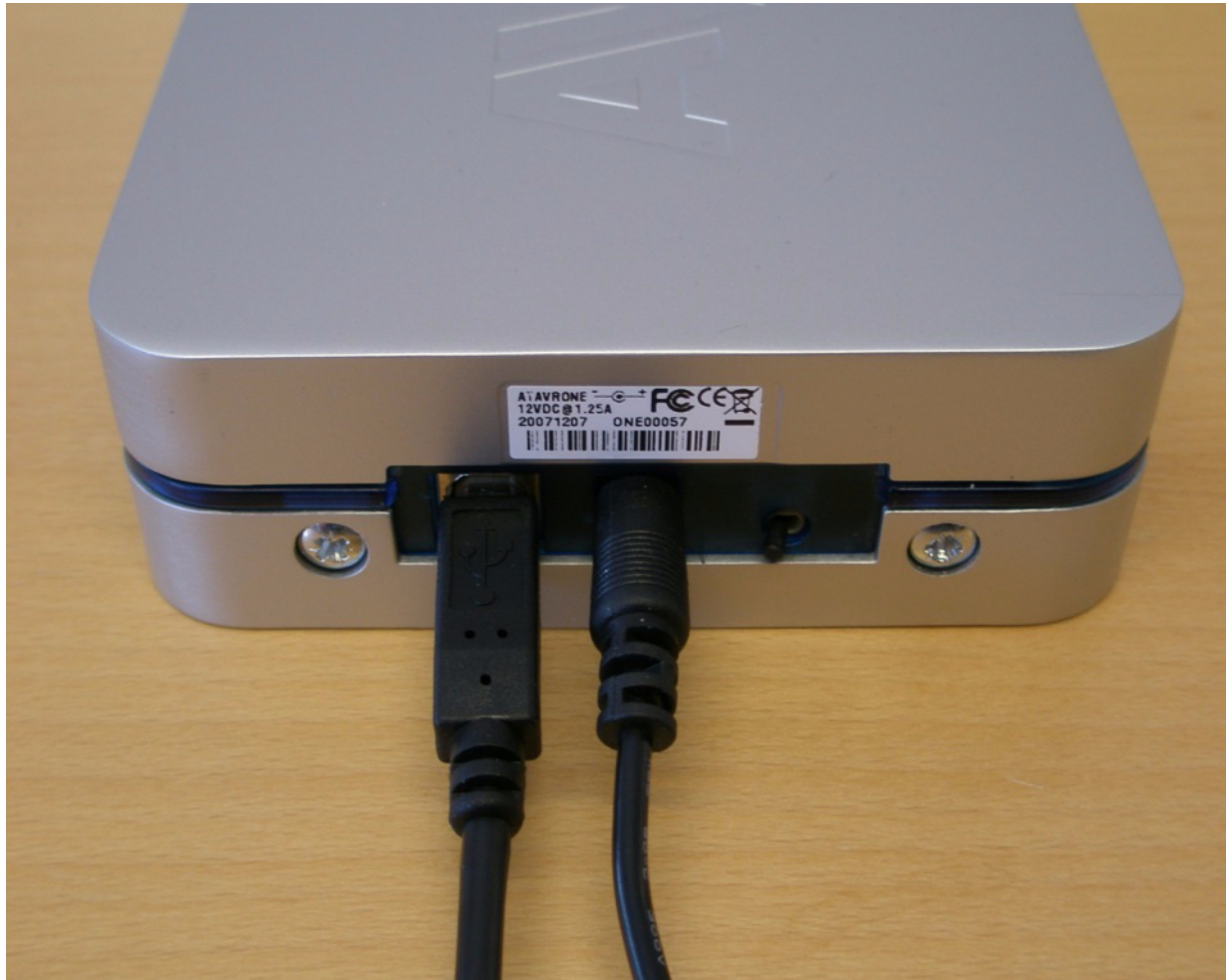
Figure 3-24. AVR ONE! connected to power and USB
