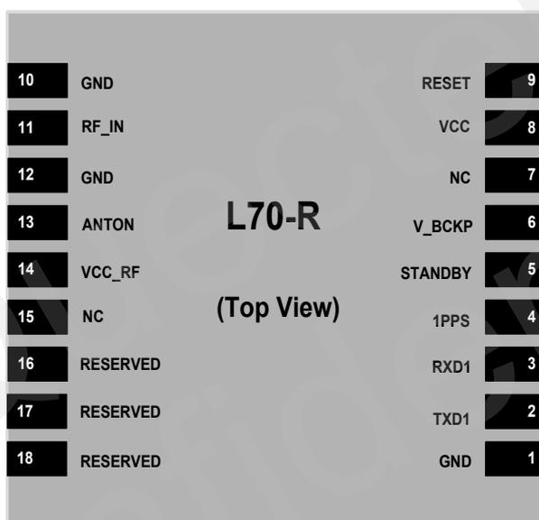
Figure 2: Pin Assignment
