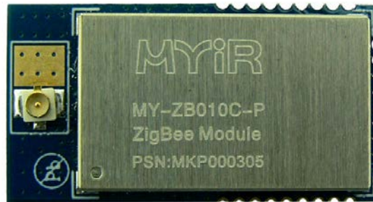
Figure 1-2 MY-ZB010C-P ZigBee Module
