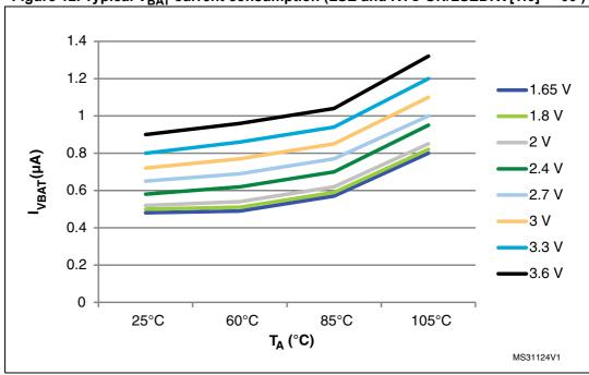
Figure 12. Typical V<sub>BAT</sub> current consumption (LSE and RTC ON/LSEDRV[1:0] = '00')
