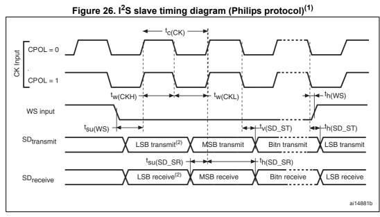
1. Measurement points are done at  $0.5V_{DD}$  and with external  $C_L$ =30 pF.
