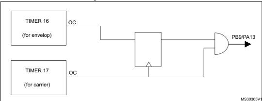
Figure 3. Infrared transmitter
