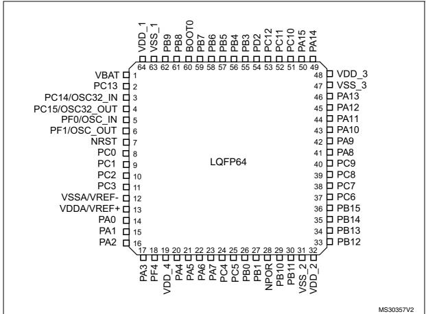
Figure 5. STM32F358xC LQFP64 pinout
