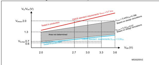
Figure 18. TC and TTa I/O input characteristics
