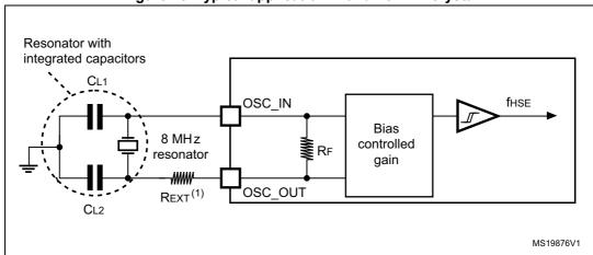
Figure 15. Typical application with an 8 MHz crystal
