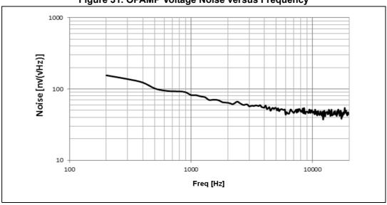
Figure 31. OPAMP Voltage Noise versus Frequency
