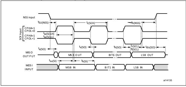
1. Measurement points are done at  $0.5V_{DD}$  and with external  $C_L$  = 30 pF.
