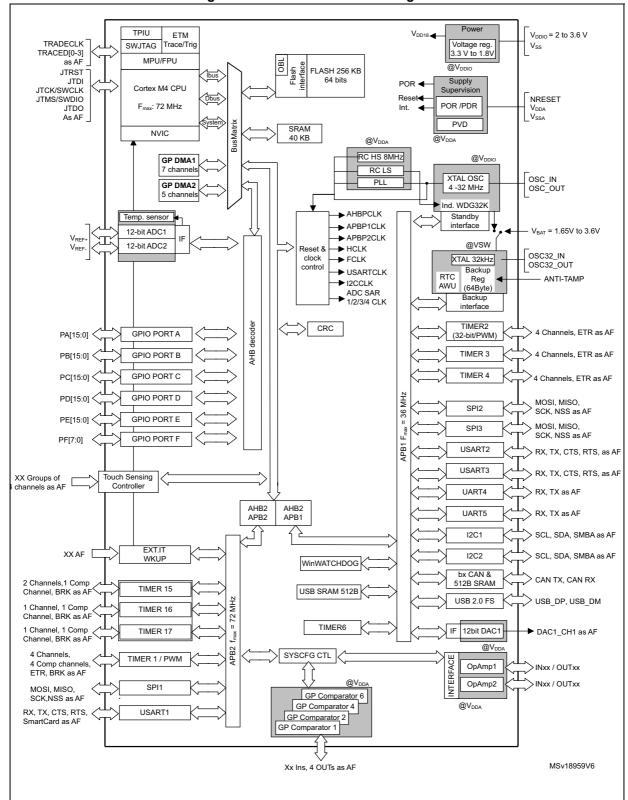
Figure 1. STM32F358xC block diagram
