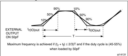
Figure 20. I/O AC characteristics definition
