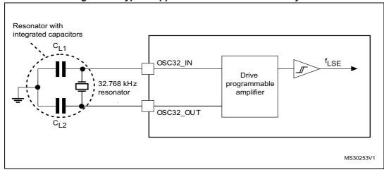
Figure 16. Typical application with a 32.768 kHz crystal
