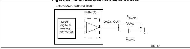
Figure 30. 12-bit buffered /non-buffered DAC
