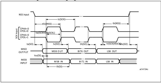
Figure 23. SPI timing diagram - slave mode and CPHA = 0
