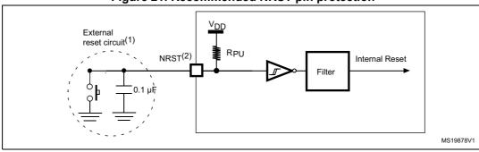
Figure 21. Recommended NRST pin protection
