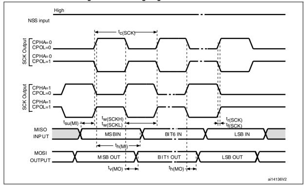
Figure 25. SPI timing diagram - master mode<sup>(1)</sup>
