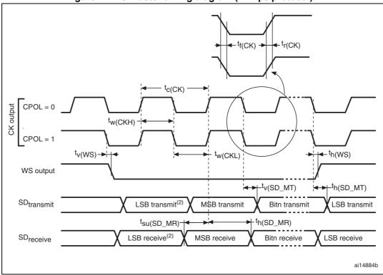
Figure 27. I<sup>2</sup>S master timing diagram (Philips protocol)<sup>(1)</sup>
