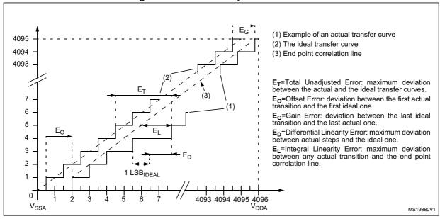
Figure 25. ADC accuracy characteristics
