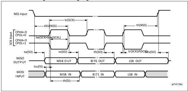
Figure 28. SPI timing diagram - slave mode and CPHA = 0
