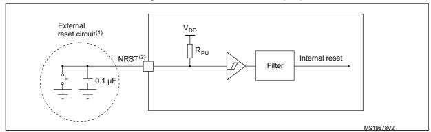
Figure 24. Recommended NRST pin protection
