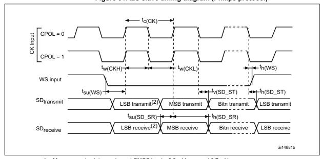
Figure 31. I2S slave timing diagram (Philips protocol)
