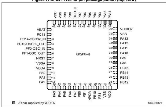
Figure 7. UFQFPN48 48-pin package pinout (top view)
