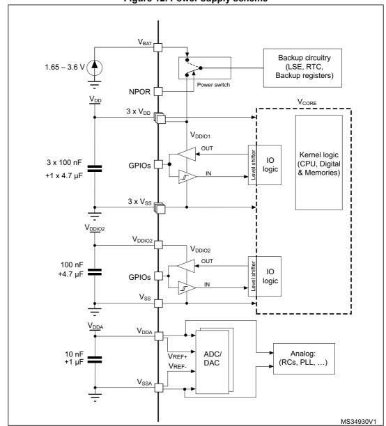
Figure 12. Power supply scheme
