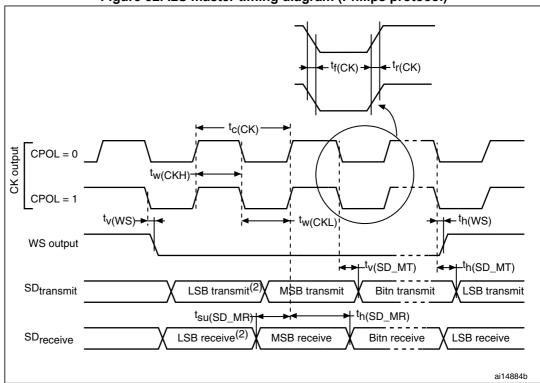
Figure 32. I2S master timing diagram (Philips protocol)
