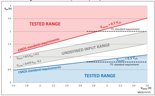
Figure 22. Five volt tolerant (FT and FTf) I/O input characteristics
