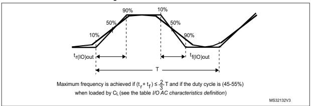
Figure 23. I/O AC characteristics definition
