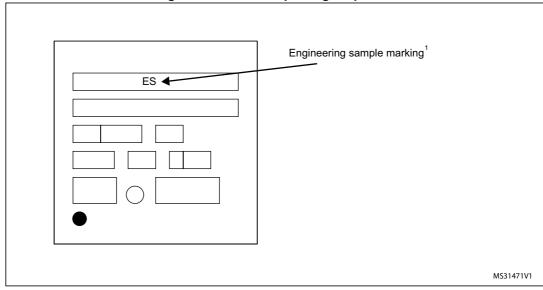
Figure 38. LQFP100 package top view
