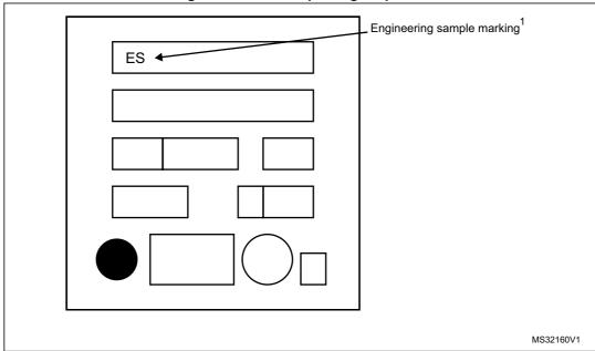
Figure 44. LQFP48 package top view
