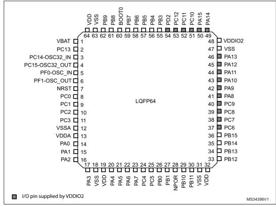
Figure 5. LQFP64 64-pin package pinout (top view)
