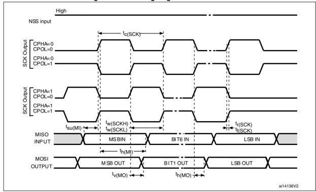
Figure 30. SPI timing diagram - master mode
