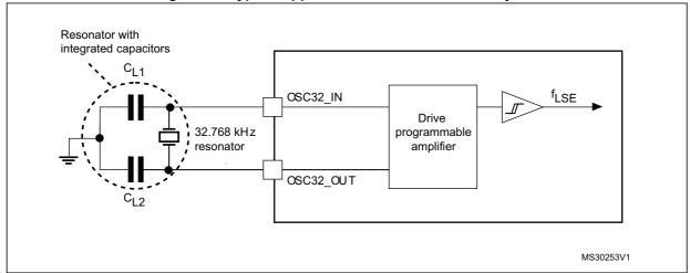
Figure 17. Typical application with a 32.768 kHz crystal
