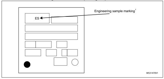
Figure 41. LQFP64 package top view
