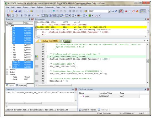
Figure 12. MDK-ARM debugger screen
