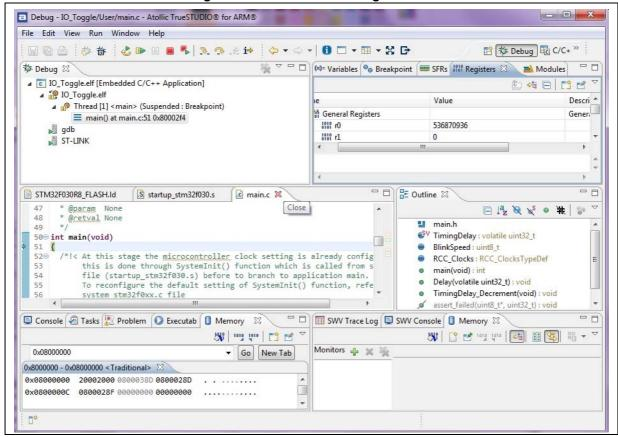
The debugger in the Atollic TrueSTUDIO can be used to debug source code at C and assembly levels, set breakpoints, monitor individual variables and watch events during the code execution.
