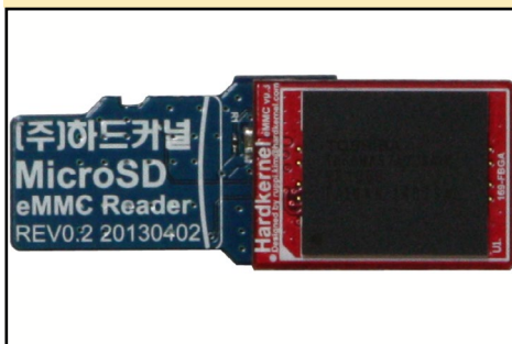
The eMMC reader attaches to the eMMC module with a small clip
