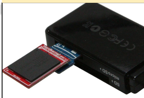
Top view of eMMC reader and eMMC module inserted into SD card reader
