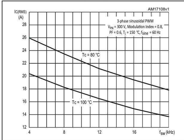
Figure 4. Maximum  $I_{C(RMS)}$  current vs.  $f_{sine}$  (1)
