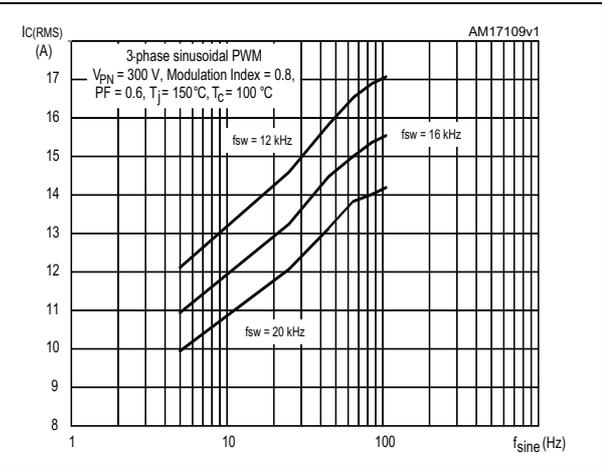
1. Simulated curves refer to typical IGBT parameters and maximum  $R_{thj-c}$ .
