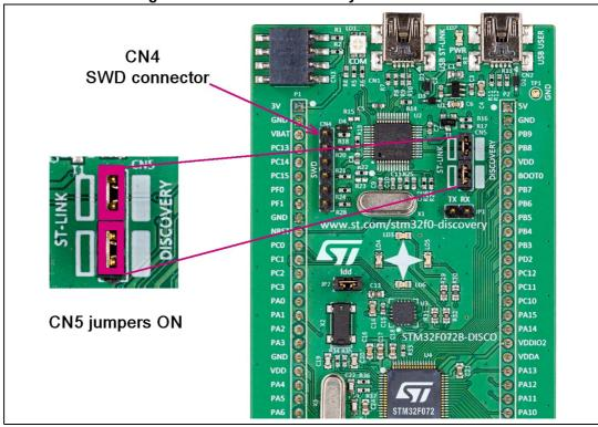
Figure 5. STM32F072 Discovery kit connections
