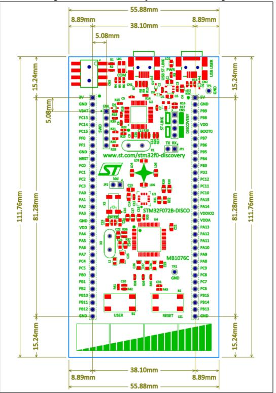
Figure 8. STM32F072 Discovery kit mechanical drawing
