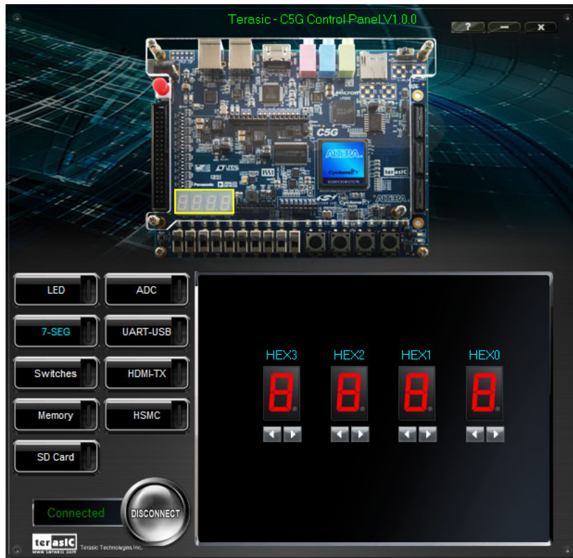
Figure 2-4 Controlling 7-SEG display
