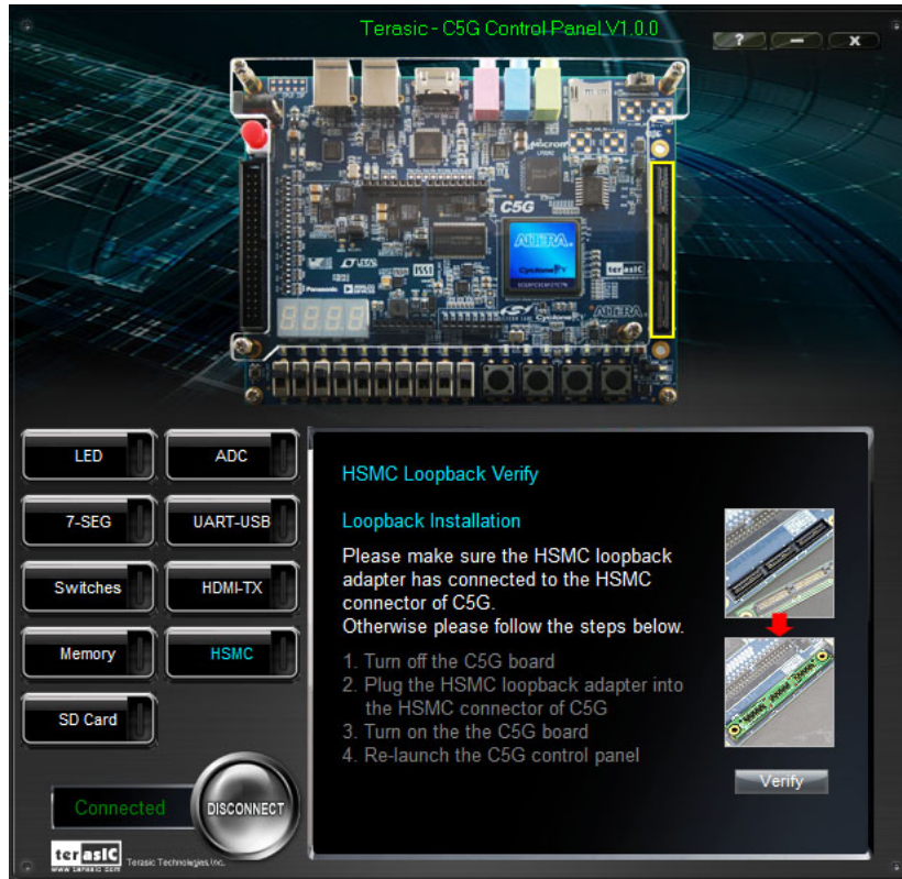
Figure 2-11 HSMC loopback verification test performed under Control Panel
