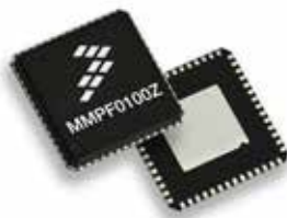
MMPF0100Z PMIC Wettable Flank Package for Automotive
