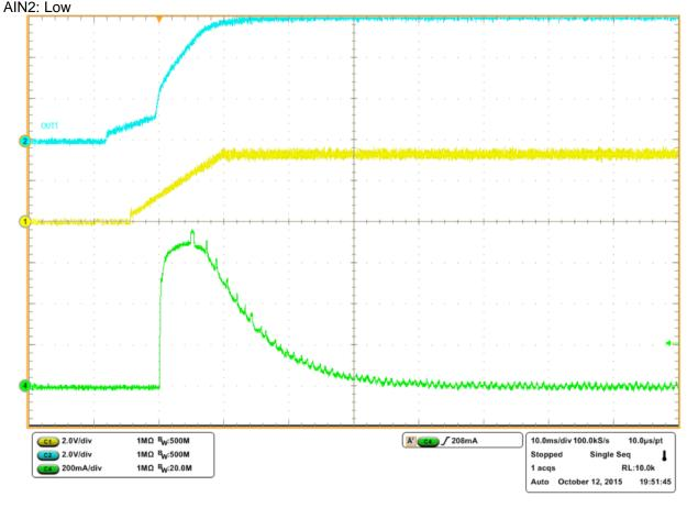
Channel 1: VM Channel 2: VCC IN1 = Logic High IN2 = Logic Low
