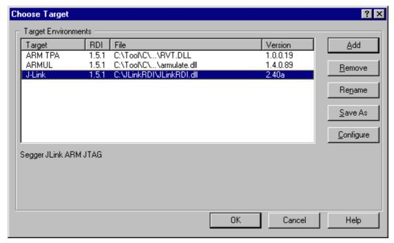
4. Select J-Link and press **OK** to connect to the target via J-Link ARM. To configure J-Link RDI refer to the chapter *Configuration* on page 41. After downloading an image to the target board, the debugger window looks as follows:
