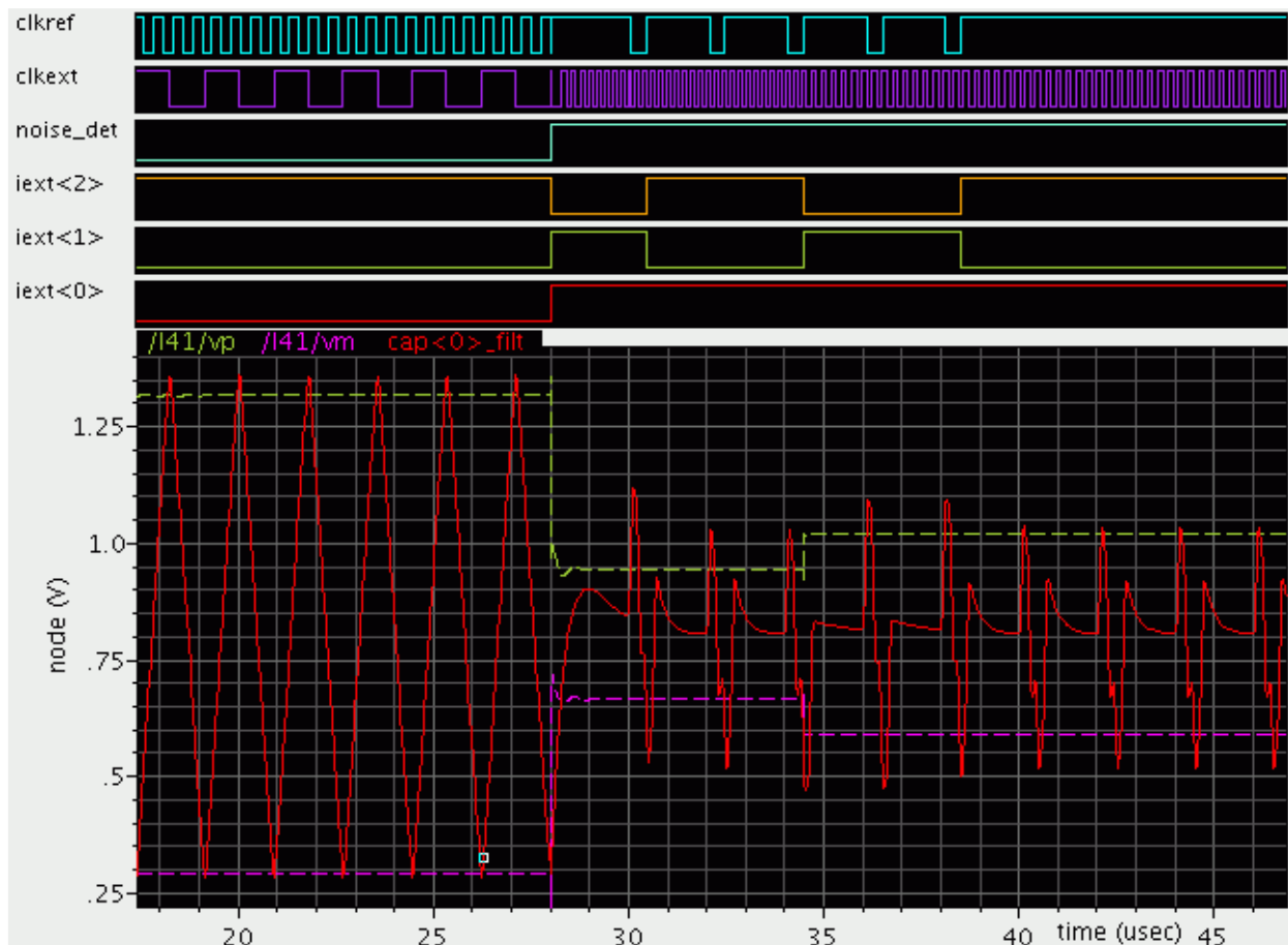
Figure 40-16. TSI noise detection mode waveform
