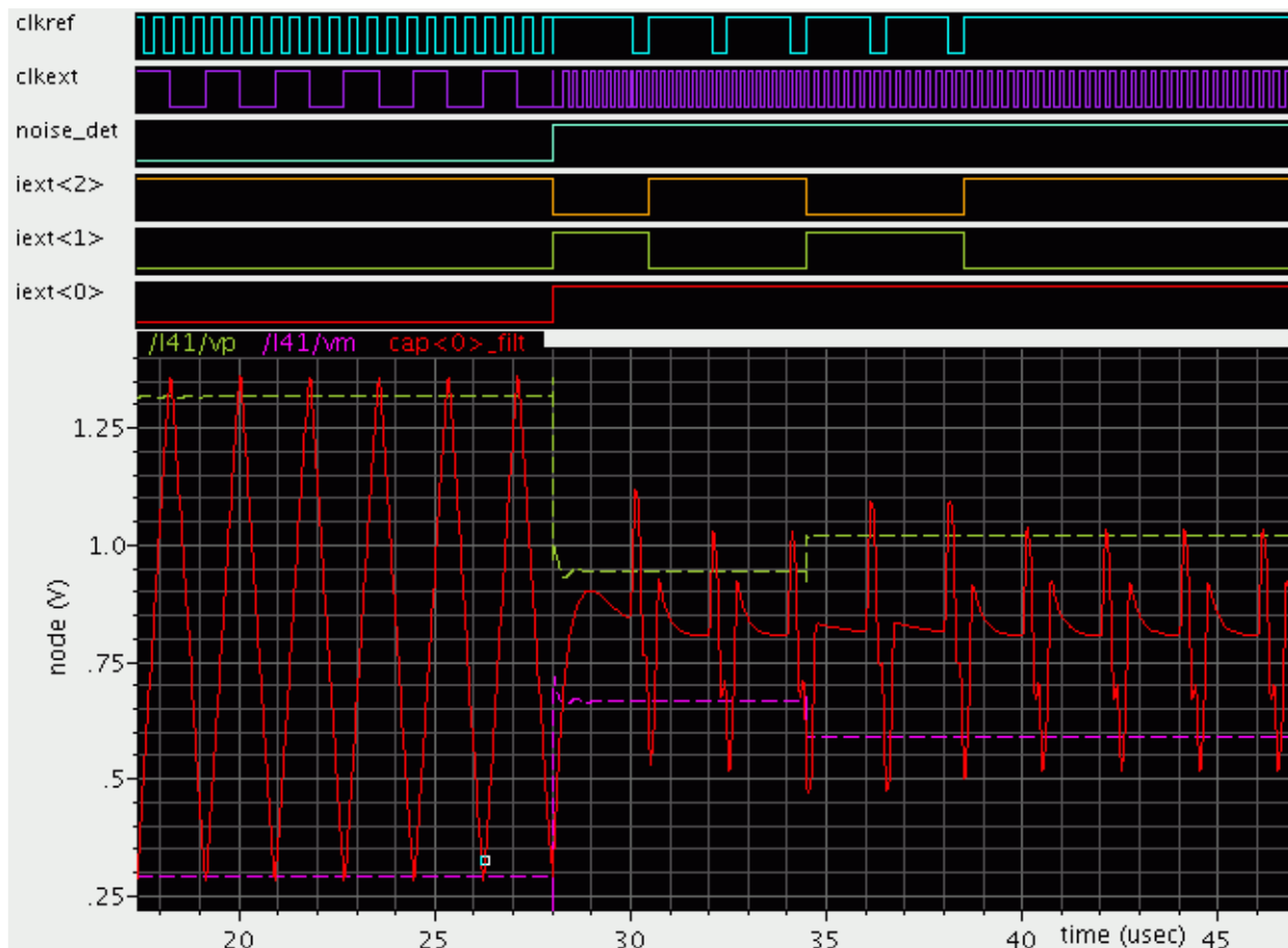
Figure 42-16. TSI noise detection mode waveform
