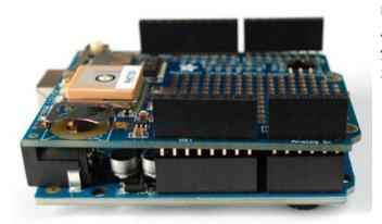
Fit the long pins through the pads until they slot into the Arduino. Depending on which version/type of Arduino you may need to use  $2 \times 8pin$  and  $2 \times 6pin$  or  $1 \times 10pin$ ,  $2 \times 8pin$  and  $1 \times 6pin$ .
