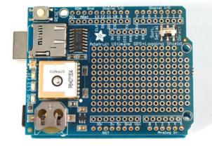
Place the shield on top so the short ends stick out thru the PCB, solder all the pins
