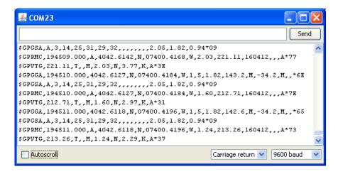
Look for the line that says \$GPRMC,194509.000,A,4042.6142,N,07400.4168,W,2.03,221.11,160412,,,A\*77 This line is called the RMC (Recommended Minimum) sentence and has pretty much all of the most useful data. Each chunk of data is separated by a comma.
