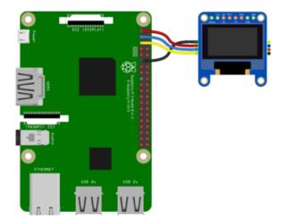
You do not need to alter the jumpers on the back - I2C is the default configuration on this display!
