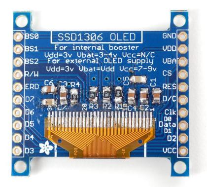
$\bullet$  VDD is the 3.3V logic power. This must be 3 or 3.3V
