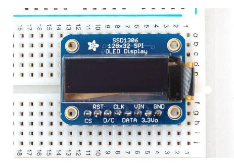
Simply connect GND to ground, and Vin to a 3 to 5V power supply. There will be a 3.3V output on the 3Vo pin in case you want a regulated 3.3V supply for something else.
