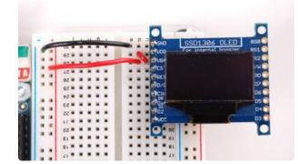
We'll be using the internal charge pump so connect VDD and VBAT together (they will connect to 3.3V). GND goes to ground.
