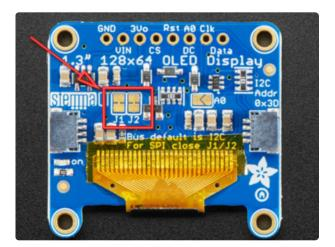
For the new STEMMA-capable version, the J1 and J2 jumpers are closed so that the display is by default in I2C mode!
