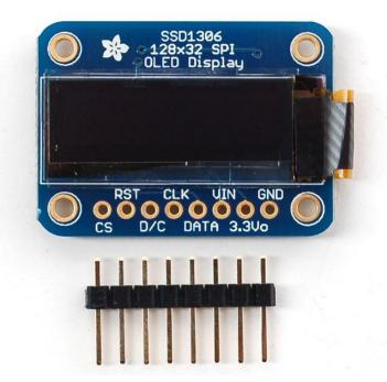
Plug the header long end down into a breadboard and place the OLED on top. Solder the short pins into the OLED PCB.
