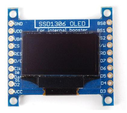
The driver chip, SSD1306 can communicate in multiple ways including I2C, SPI and 8bit parallel. However, only the 128x64 display has all these interfaces available. For the 128x32 OLED, only SPI is available. Frankly, we prefer SPI since its the most flexible and uses a small number of I/O pins so our example code and wiring diagram will use that.
