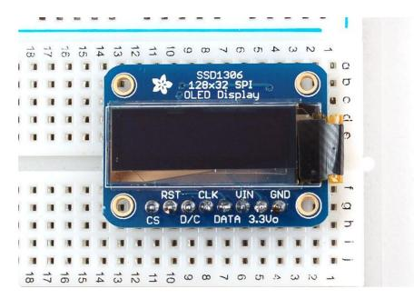
Finally, connect the pins to your Arduino - GND goes to ground, Vin goes to 5V, DATA to digital 9, CLK to digital 10, D/C to digital 11, RST to digital 13 and finally CS to digital 12.
