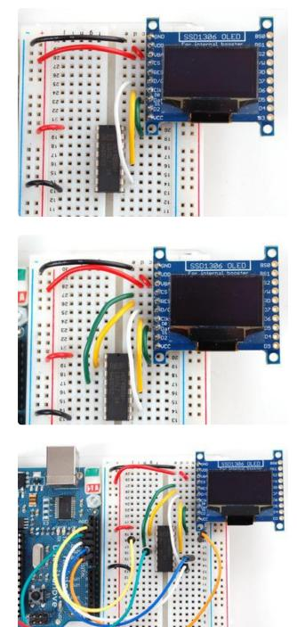
Connect pin 10 to D/C pin 12 to CLK (SPI clock) and pin 15 to DAT (SPI data).
