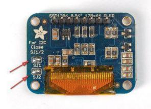
If you have the older non-STEMMA version of the OLED, you'll need to solder the two jumpers on the back of the OLED. Both must be soldered 'closed' for I2C to work!
