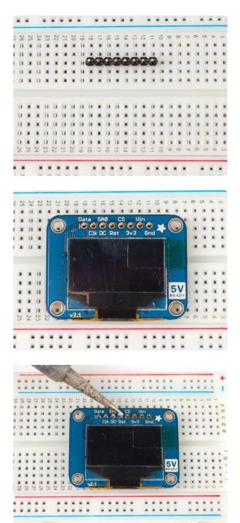
Start by placing an 8-pin piece of header with the long ends down into a breadboard for stability
