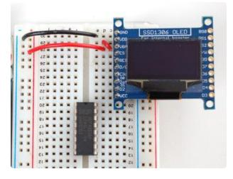
Place a CD4050 level shifter chip so pin one is at the top.
