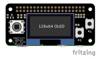
• The OLED Bonnet comes fully assembled. Simply plug into the Raspberry Pi as shown.
