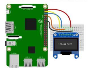
You must solder two jumpers closed on the back of the display to use with I2C!
