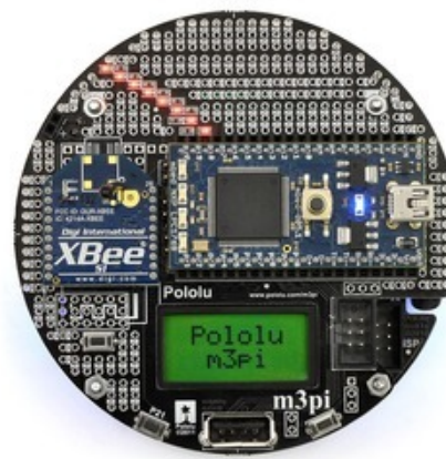
Pololu m3pi robot with mbed and XBee modules socketed.
