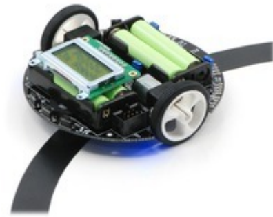
Pololu 3pi robot on a 3/4" black line.
