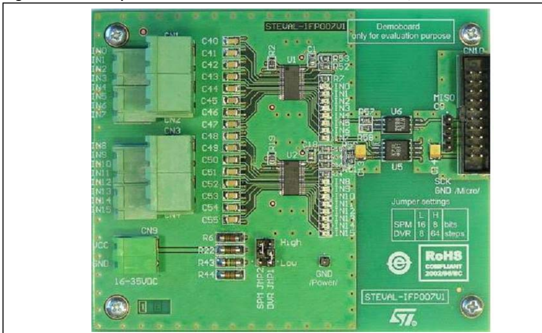
Figure 5. 8/16 input channel current limiter based on SCLT3-8, STEVAL-IFP007V1
