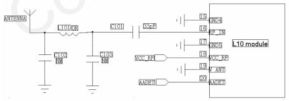
Figure 12: Reference design for passive antenna
