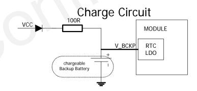
Figure 6: Reference charging circuit for chargeable battery
