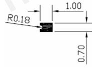
Figure 18: PAD Bottom dimensions (Unit:mm)
