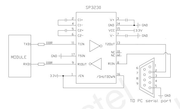
Figure 9: RS-232 level shift circuit
