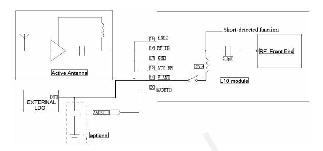
Figure 15: Active antenna with external LDO
