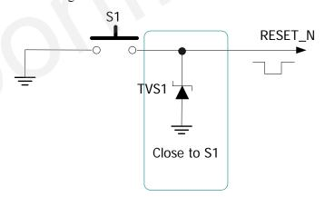
Figure 3: Reference reset circuit using button
