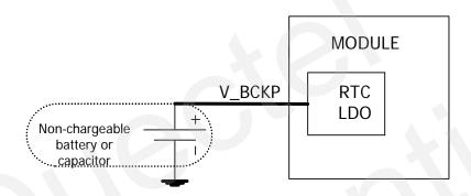
Figure 5: RTC supply from non-chargeable battery or capacitor
