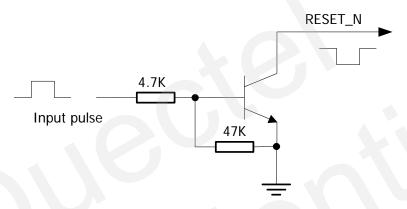
Figure 2: Reference reset circuit using OC circuit
