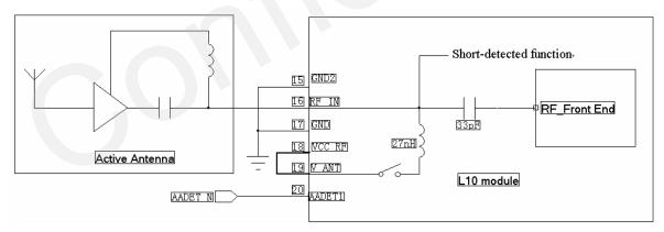
Figure 14: Active antenna with VCC\_RF
