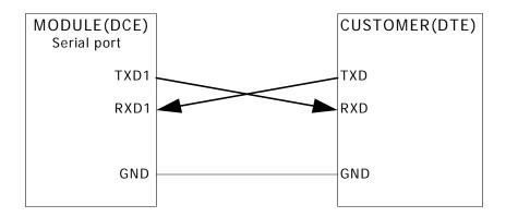
**Figure 8: Connection of serial interfaces**
