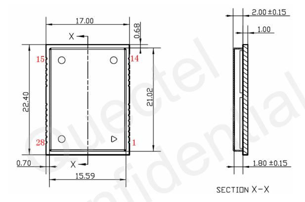
Figure 16: L10 Top view and Side dimensions (Unit:mm)
