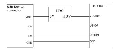
Figure 10: USB interface circuit
