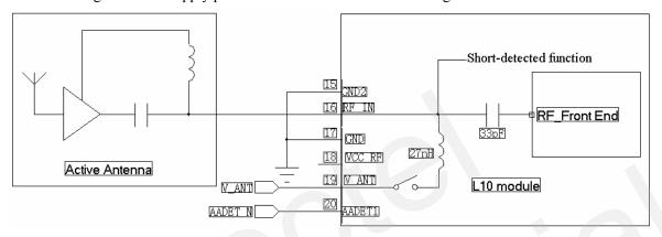
Figure 13: Active antenna biasing
