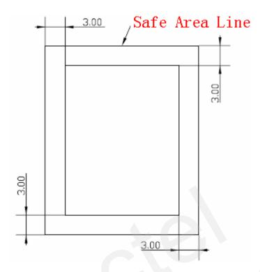
Figure 19: Footprint of recommendation (Unit:mm)
