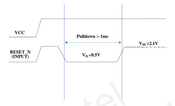
Figure 4: Timing of restart system
