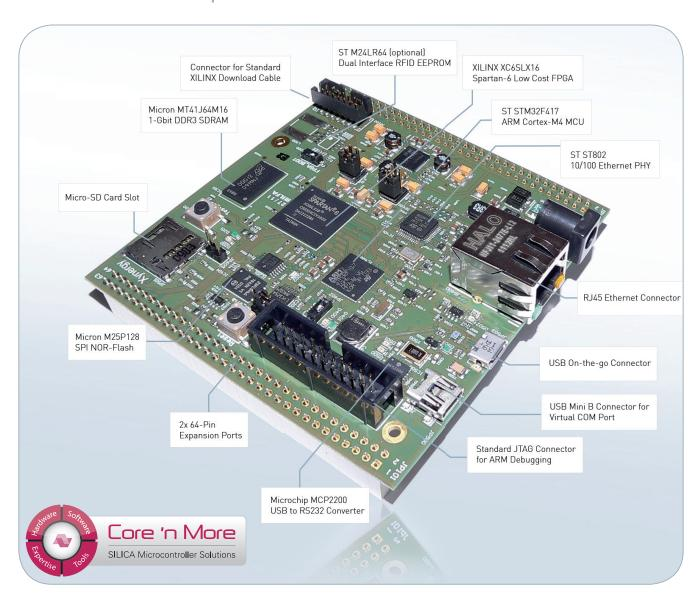
The Silica Xynergy-M4 Board combines an ARM Cortex-M4 based STMicroelectronics STM32F417 controller with a Xilinx Spartan-6 low-cost FPGA (XC6SLX16) in one design.
