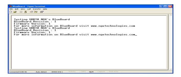
UART0 can also be used for serial programming. If the selected bootloader mode is Manual then Half modem cable should be used, else if it is in Auto mode use full modem cable. Note that after programming in auto mode the serial cable should be disconnected.
