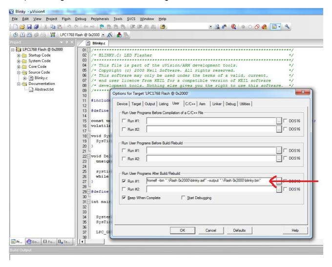
Insert the user command in Run #1 ticking the check box. After compile and build the entire project, from elf it creates hex file along with the hex file there will be another file with the extension .axf. This user command is used to convert .axf file to .bin. Here in fig. Above blinky.axf is converted to blinky.bin which is used for drag drop programming with the USB boot-loader that allows you to enumerate the board as a Mass Storage Device.
