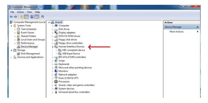
Connect the USB cable to USB connector. The USB enumeration can be checked in device manager. The mX-LPC1768-S enumerates as a USB HID as shown in the fig above.
