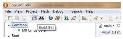
After building the project initiate debug to download the program to the target. Press F5 to run the program execution. This blinks the D2 on mX-LPC1114-S board.
