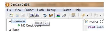
After building the project initiate debug to download the program to the target. Press F5 to run the program execution. This blinks the D2 on mX-LPC1343-S board.
