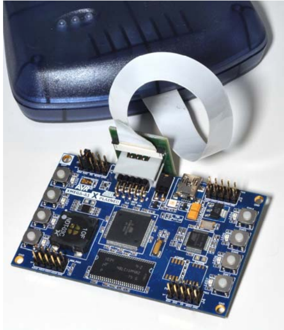
Figure 4-2. Connecting the AVR JTAGICE mkII probe to an Xplained board.
