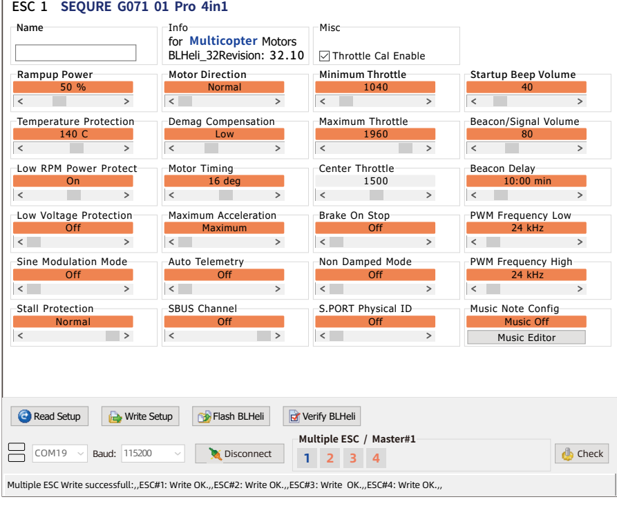
BLHeli_32 firmware visual programming parameter adjustment interface(pre-release)
