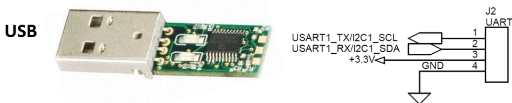
Figure 9. UART TX/RX (3v3 level)
