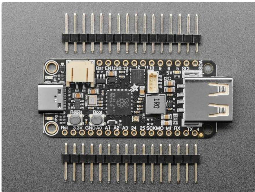
At the Feather's heart is an RP2040 chip, clocked at 133 MHz and at 3.3V logic, the same one used in the [Raspberry Pi Pico \(http://adafru.it/4864\)](http://adafru.it/4864). This chip has 264K of RAM and is paired with a whopping 8MB of external QSPI FLASH! There's even room left over for a STEMMA QT connector for plug-and-play of I2C devices!
