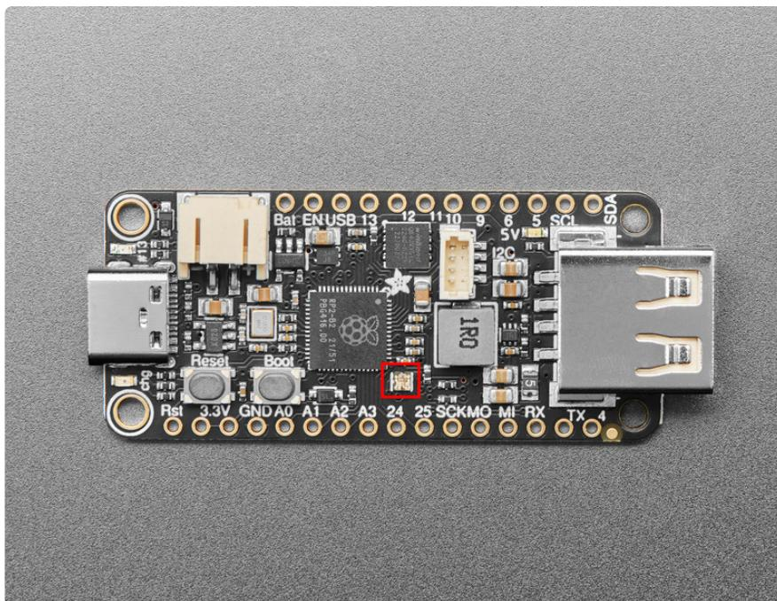
The **NeoPixel LED** is located above the D24 and D25 pin labels.
