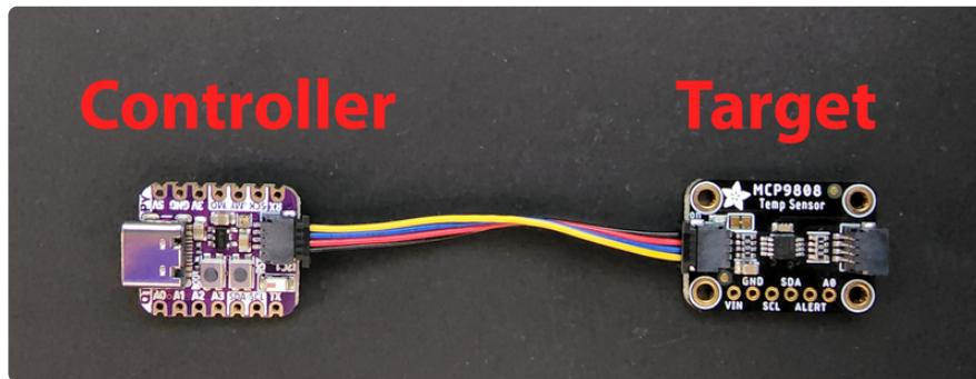
The **I2C**, or [inter-integrated circuit](https://adafru.it/u2a) (<https://adafru.it/u2a>), is a 2-wire protocol for communicating with simple sensors and devices, which means it uses two connections, or wires, for transmitting and receiving data. One connection is a clock, called **SCL**. The other is the data line, called **SDA**. Each pair of clock and data pins are referred to as a **bus**.
