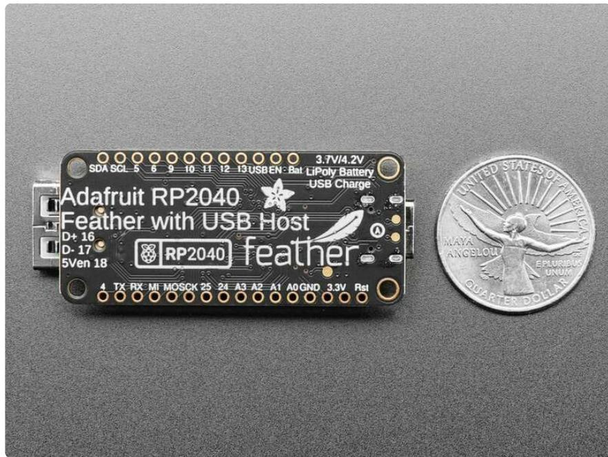
To make it easy to use for portable projects, we added a connector for any of our 3.7V Lithium polymer batteries and built-in battery charging. You don't need a battery, it will run just fine straight from the USB Type C connector. But, if you do have a battery, you can take it on the go, then plug in the USB to recharge. The Feather will automatically switch over to USB power when it's available.
