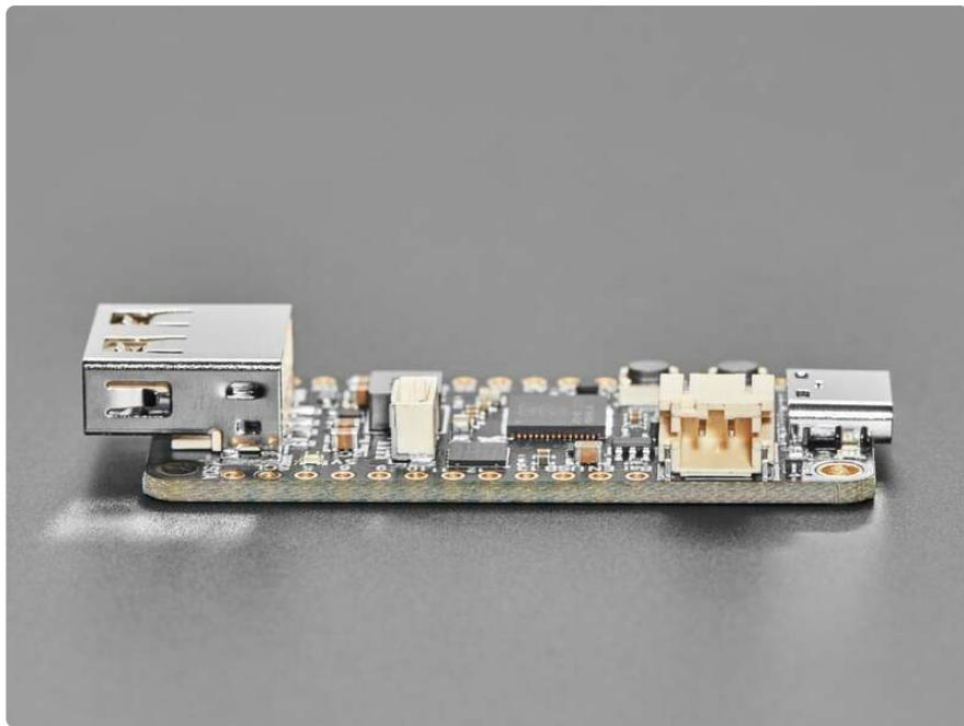
[We also include a 1 Amp boost converter based on the TPS61023 \(http://adafru.it/4654\)](http://adafru.it/4654) so you can run from Lipo battery and get a nice clean 5V output for the USB devices. The booster has the enable pin tied to one of the extra GPIO on the RP2040 so power can be manually turned on and off to hard-reset whatever is connected.
