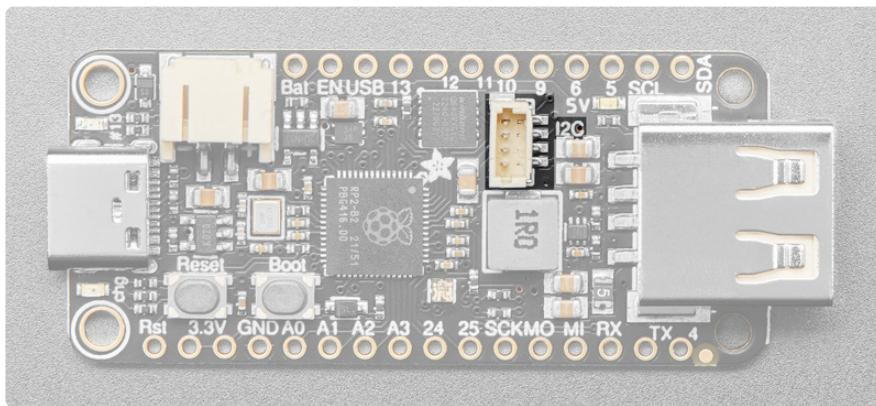
In the middle of the board, to the left of the USB A connector, is the **STEMMA QT connector**! This means you can connect up [all sorts of I2C sensors and breakouts](https://adafru.it/18fV) (<https://adafru.it/18fV>), no soldering required! This connector uses the SCL and SDA pins for I2C, which end up being the RP2040's I2C1 peripheral. In CircuitPython, you can initialise the STEMMA connector with `board.STEMMA_I2C()` (as well as with `board.SCL` `board.SDA`). In Arduino it is `Wire`.
