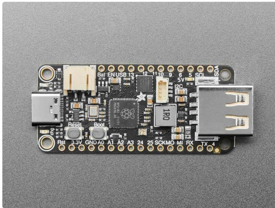
You're probably really used to microcontroller boards with USB, but what about a dev board with two? Two is more than one, so that makes it twice as good! And the **Adafruit Feather RP2040 with USB Host** is double-the-fun of our other Feather RP2040 boards, with a USB Type A port on the end for connecting USB devices to.
