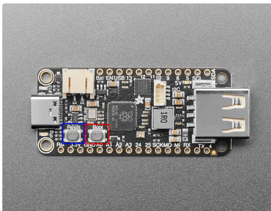
To enter the bootloader, hold down the **BOOT/BOOTSEL button** (highlighted in red above), and while continuing to hold it (don't let go!), press and release the **reset button** (highlighted in red or blue above). **Continue to hold the BOOT/BOOTSEL button until the RPI-RP2 drive appears!**
