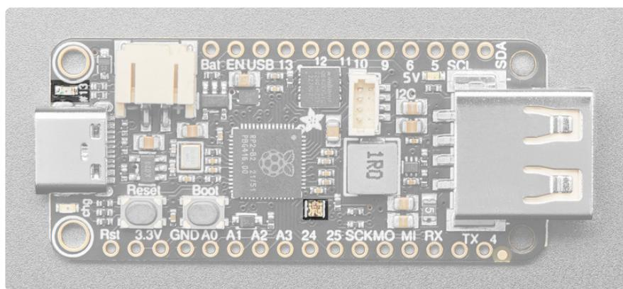
Above the pin labels for D24 and D25 is the status **NeoPixel LED**. It is connected to **GPIO21**. In CircuitPython, the NeoPixel is available at `board.NEOPIXEL` and the library for it is available in [the bundle](https://adafru.it/ENC) (<https://adafru.it/ENC>). In Arduino, it is accessible at `PIN_NEOPIXEL`. The NeoPixel is powered by the 3.3V power supply but that hasn't shown to make a big difference in brightness or color. In CircuitPython, the LED is used to indicate the runtime status.
