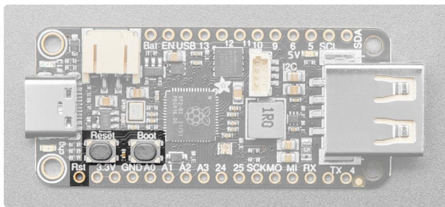
The **Boot button** is the button on the right, located on **GPIO7**. It is available as `board.BUTTON` in CircuitPython, and is available for use in Arduino as `PIN_BUTTON`. It is also used to enter the bootloader. To enter the bootloader, press and hold Boot and then power up the board (either by plugging it into USB or pressing Reset). The bootloader is used to install/update CircuitPython.
