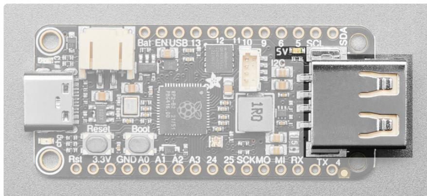
On the right end of the board is a USB type A port for connecting USB devices to. The RP2040 has a PIO peripheral that can be used to emulate a USB host. This USB-A port can be used for sending or receiving data from an attached USB device.
