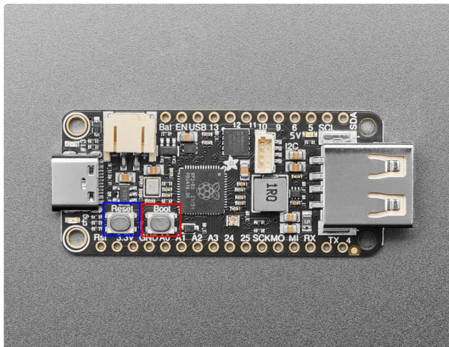
To enter the bootloader on this Feather, hold down the **Boot button** (highlighted in red above), then press the **Reset button** (highlighted in blue above). **Continue holding the Boot button until the RPI-RP2 drive appears!** Then release the Boot button. The board is now in the bootloader!
