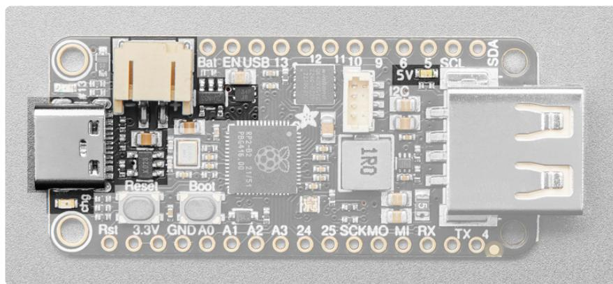
The above shows the **USB C connector** (left center), the **chg LED** (below the USB C connector), the **LiPoly JST connector** (top left), the **5V LED** (behind the USB-A port), as well as the changeover diode (to the right of the JST jack), the 3.3V regulators (to the left of the JST connector and the USB C connector), the 5V boost converter and the charging circuitry (below the JST connector).
