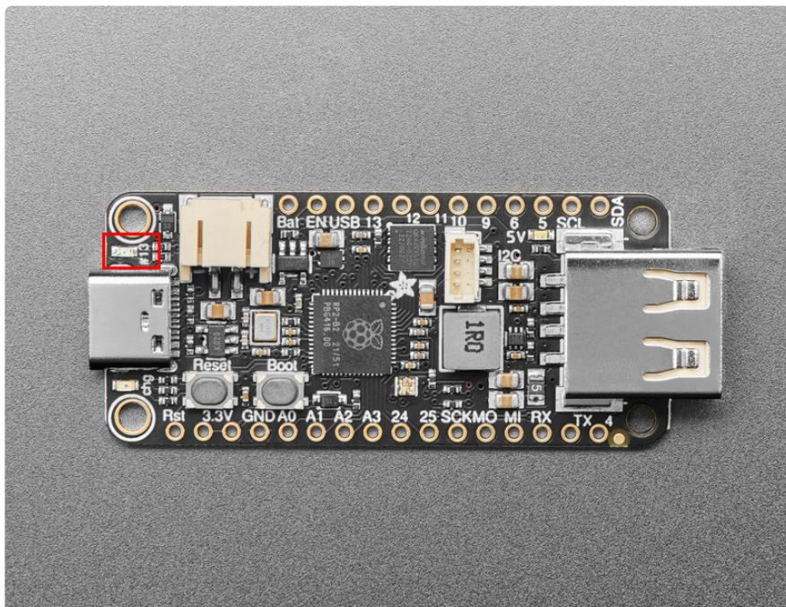
The red LED is above the USB-C connector on the left side of the board.
