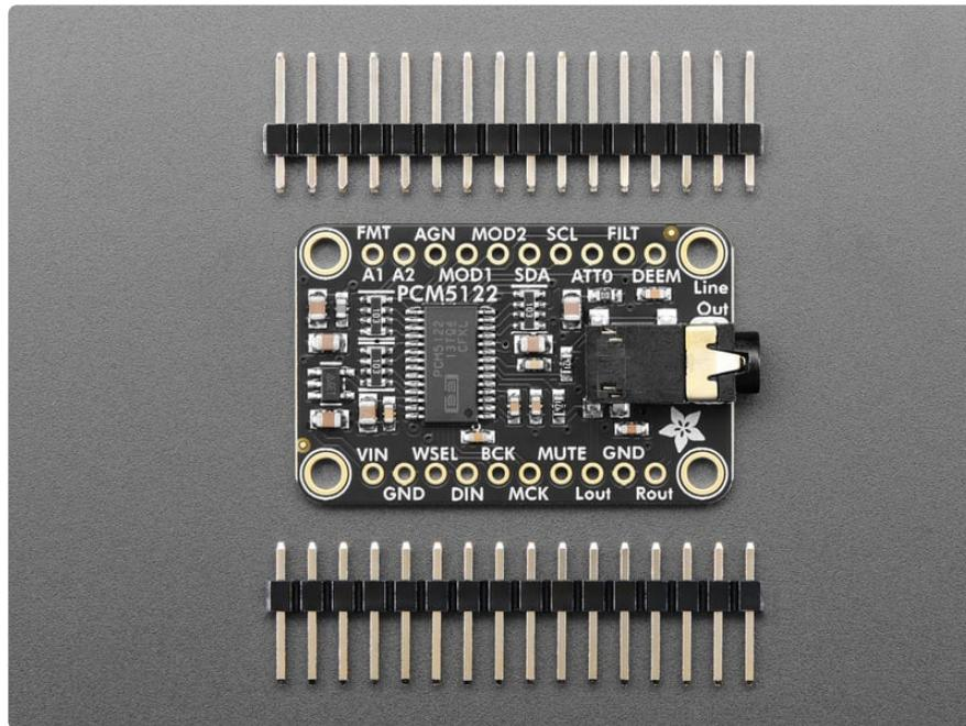
The audio outputs are also available on breakout pads if you want to wire directly without using the 3.5mm jack. Audio output is not AC-coupled because it is centered on ground: you can plug it into anything that is either AC coupled or has the same ground reference. Note that this is a line-level output, it cannot drive headphones - the output is for no less than 1K ohm loads!
