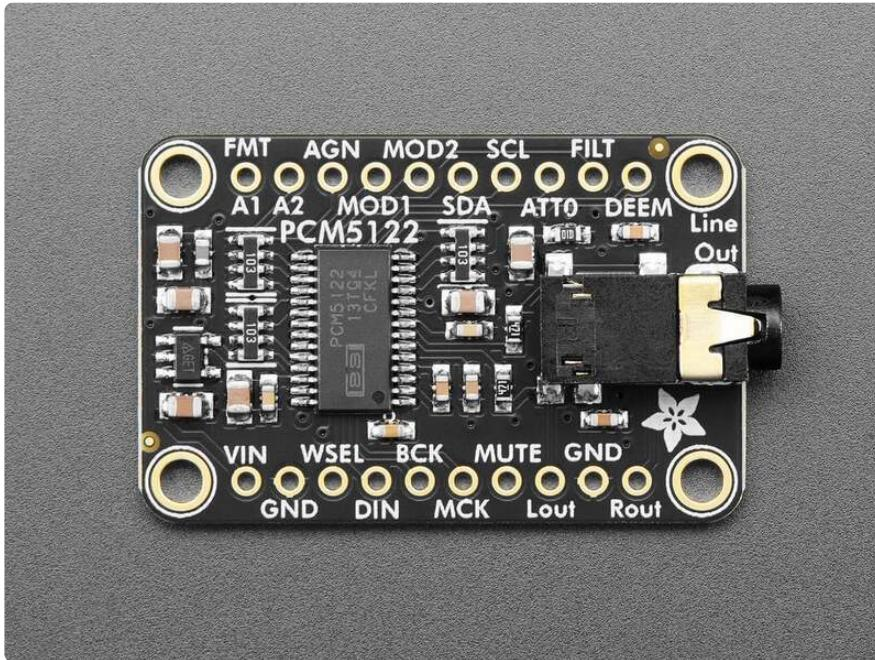
For converting digital I2S audio from your ESP32/RP2350 or Raspberry Pi, you'll need a digital-to-analog-converter (DAC). And the **Adafruit PCM5122 I2S DAC** is both powerful and easy to use - with excellent audio quality! It's got clean, high-quality, stereo audio and does not need any MCLK signal, or I2C configuration. Literally just pipe some I2S audio in and it'll just work.
