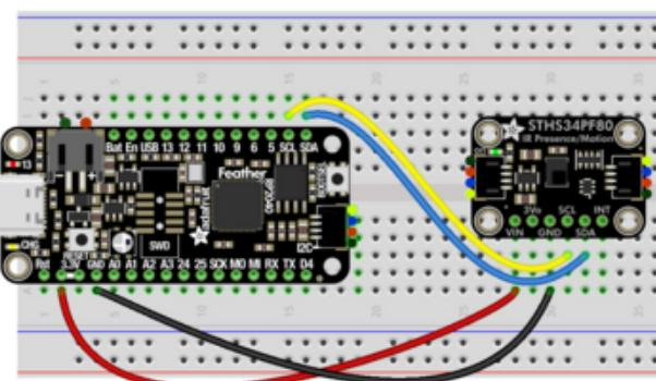
Board 3V to breakout VIN (red wire)
