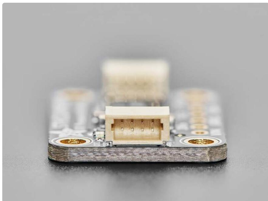
Nice sensor right? So we made it easy for you to get right into your next project. The surface-mount sensor is soldered onto a PCB and comes with a 3.3V regulator and level shifting so you can use it with a 3V or 5V logic microcontroller or single board computer without worry.
