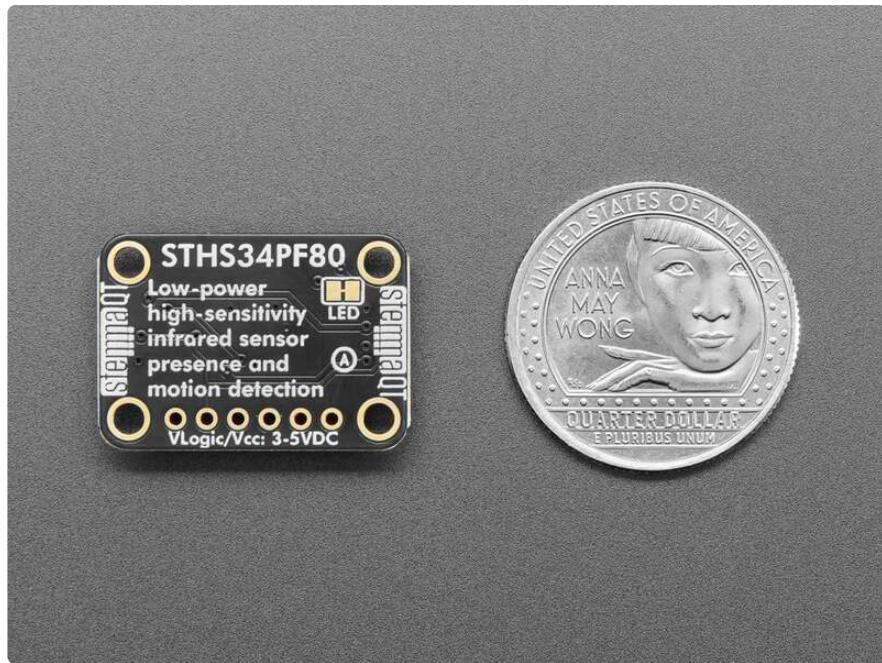
The Adafruit STHS34PF80 IR Presence / Motion Sensor is like a deluxe version of the classic PIR sensor in that it has an IR sensing element that works up to 4 meters away and doesn't require a lens, which makes it easier to integrate into small enclosures. It also comes with a full I2C interface so you can get detailed information about how much IR was detected, and whether there's presence, movement, or temperature changes.
