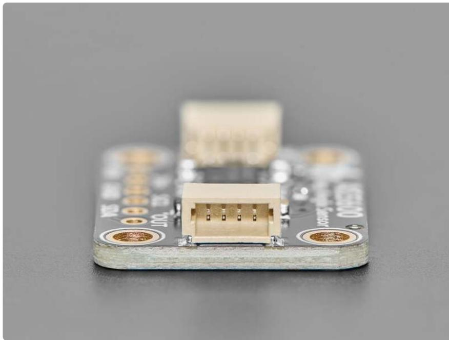
Comes as a fully assembled breakout board a small bit of header. Some light soldering is required to attach the header for use on a breadboard.
