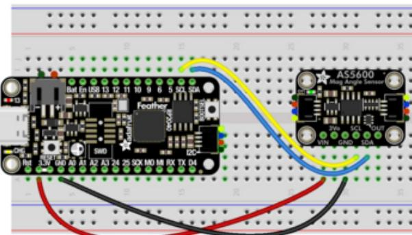
Board 3V to breakout VIN (red wire)
