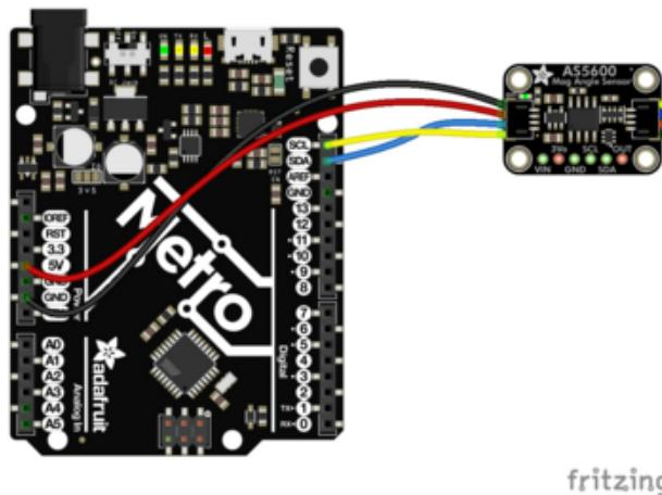
Board 5V to breakout VIN (red wire)
