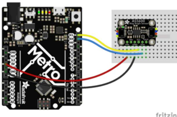
Board 5V to breakout VIN (red wire)
