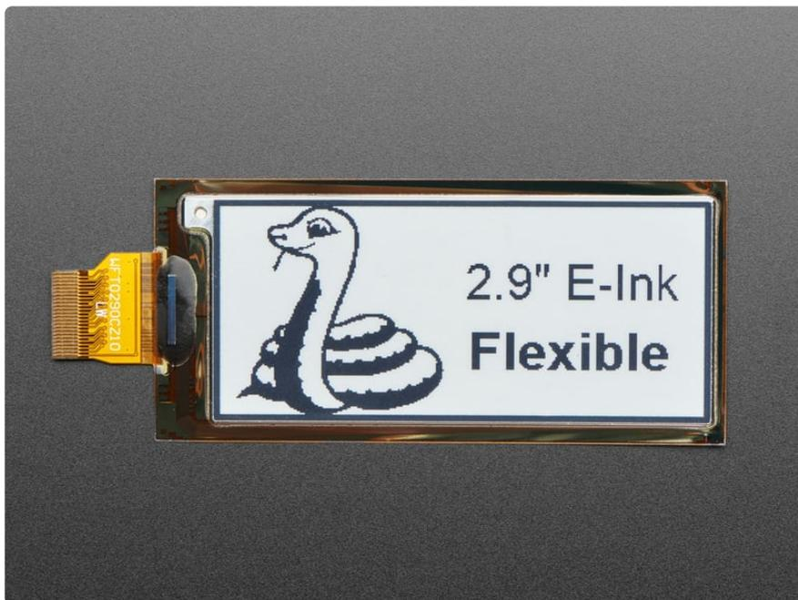
Using our Arduino library, you can create a 'frame buffer' with what pixels you want to have activated and then write that out to the display. Most simple breakouts leave it at that. But if you do the math,  $296 \times 128 \text{ pixels} \times 2\text{-bits-per-pixel} = 9.5 \text{ KBytes}$ . Which won't fit into many microcontroller memories. Heck, even if you do have 32KB of RAM, why waste 9KB?
