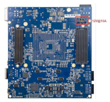
Figure 1-7 Power connector for connecting based board
