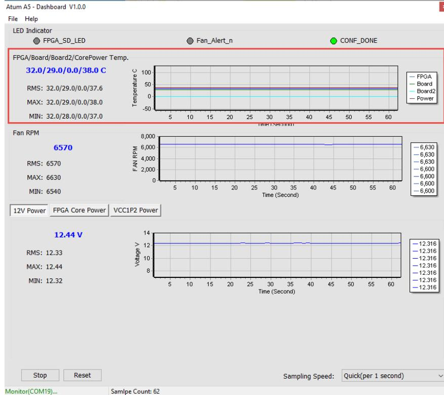
Figure 3-9 Temperature section
