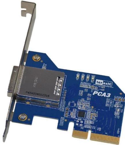
Figure 2-32 PCIe Cabling Adaptor(PCA) Gen 3 card
