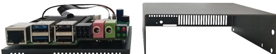
6. Use a screwdriver to loosen 6 screws of PCBA mounting counterclockwise and remove the bottom cover.
