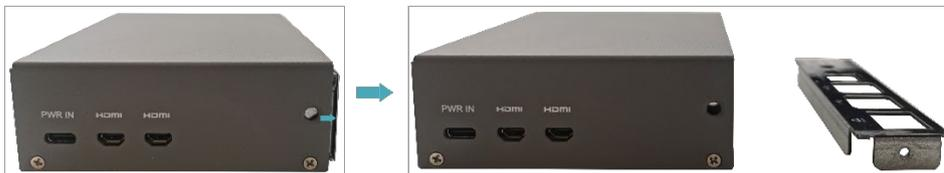
4. Use a screwdriver to loosen four M2.5 screws and one grounding screw on two sides counterclockwise, as shown in the red mark in the figure below.
