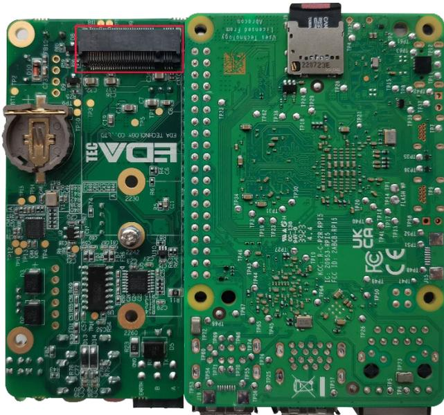
4. Use a screwdriver to loosen the screws that secure the SSD counterclockwise.
