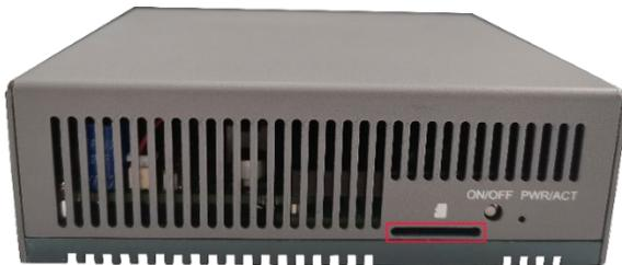
2. Insert the SD card into the corresponding card slot with the contact side facing up, making sure it will not fall out.
