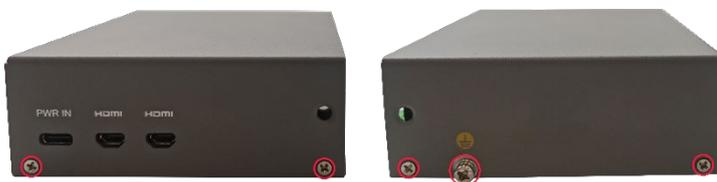
5. Remove the upper cover upward.
