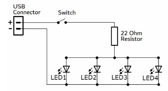
The circuit diagram for the 5V LED Desk Lamp is shown above. It is a very simple circuit. The board contains a switch, four LEDs all sharing a current limit resistor.
