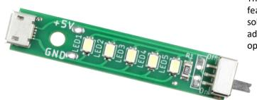
The board also features +5V & GND solder pads, for additional powering options.
