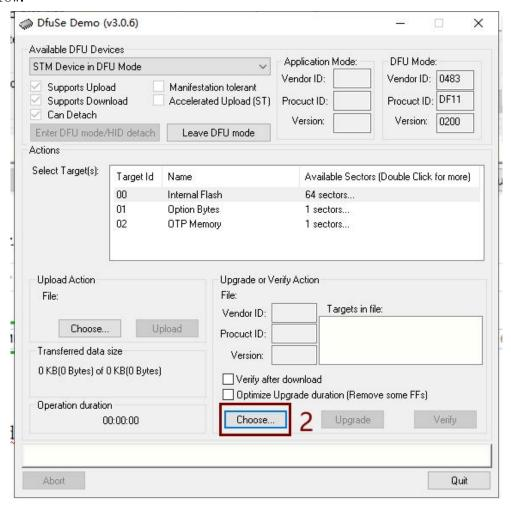
4. Select the downloaded firmware file "canable2-b158aa7.dfu", as shown in Figure 3 below.
